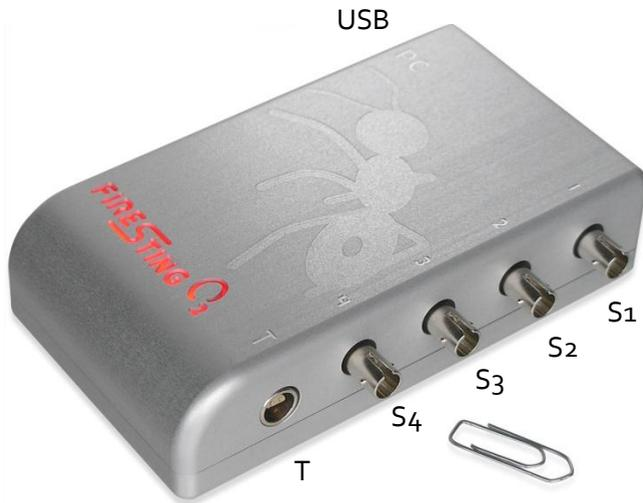
Depending on the purchased version, the *Firesting O<sub>2</sub>* is equipped with 1, 2, or 4 channels (receptacles S1 to S4) for fiber-optic oxygen sensors and one receptacle (T) for a temperature sensor. The USB-connector provides the energy supply and the data exchange with the PC. The device is operated by the Windows software *Firesting Logger* provided by *Pyro Science*.
